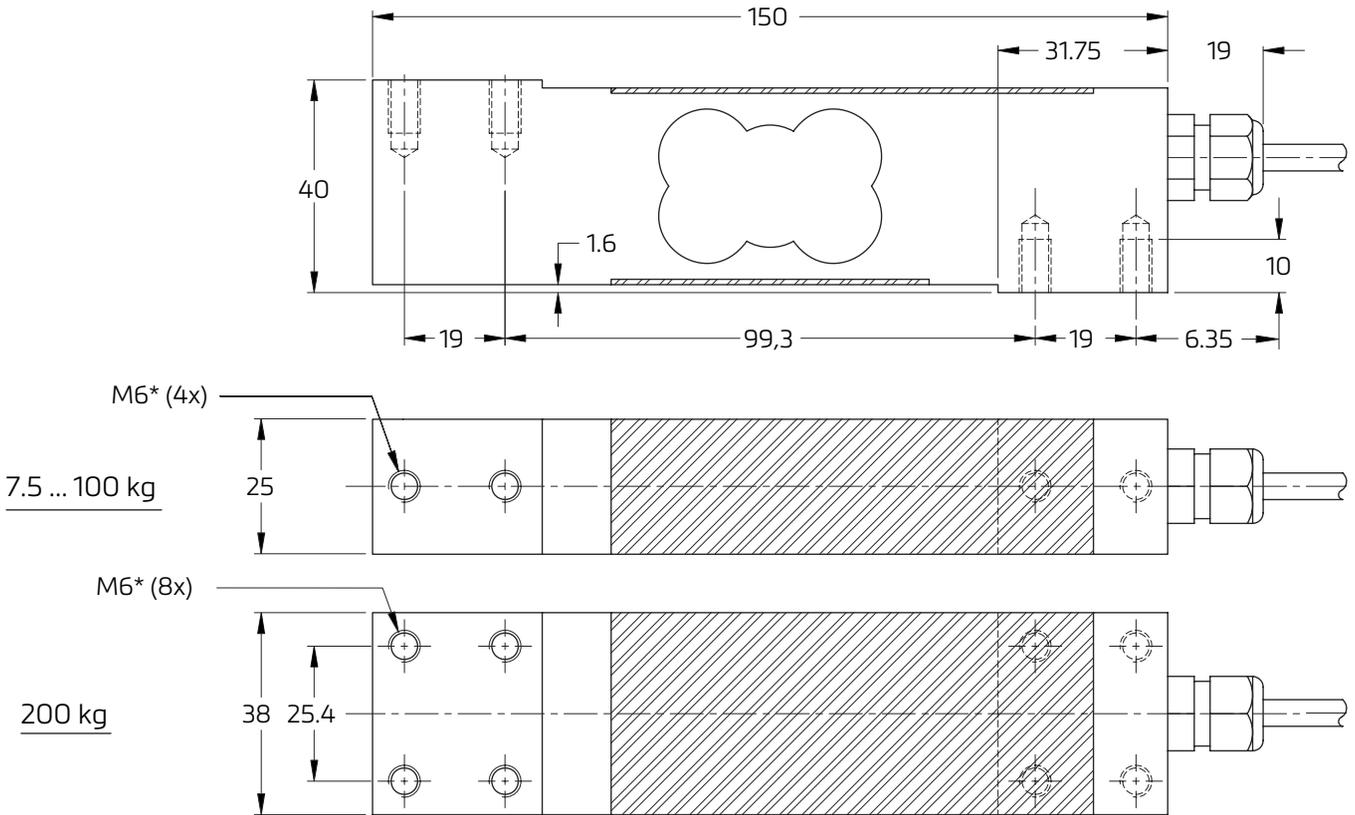
PC1: Mounting bolts M6 8.8; torque 10 Nm. Torque value assumes oiled threads.
