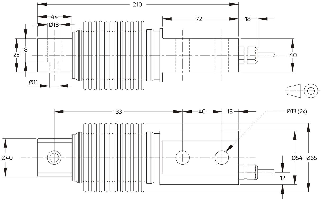
Mounting bolts M12 8.8; torque 90 Nm. Torque value assumes oiled threads.
