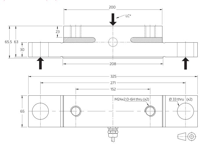
Recommended torque for mounting bolts: 1,030...1,140Nm. Torque value assumes oiled threads. Note: Holes, recesses, cutouts and radii are identical on both sides of the load cell. LC\* - Load centre
